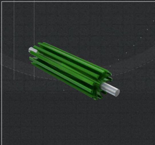
Fluent Conveyors offers Winged pulleys in CEMA, Mine, and Super Duty classes. Winged pulleys help to remove material from the back side of the belt and minimize cleaning and down time. Fluent winged pulleys can also be had with a chevron pattern wing to increase the removal of unwanted material.
