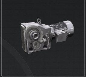
The helical bevel gearmotors can be had in single stage or two stage as well as cast steel housing or aluminum housing. These compact and powerful drive systems can come in various stages of carrion resistance and offer torques from 1,593lb-in to 442,500lb-in. The helical bevel gearmotors have many options including foot mounted, torque arm moutned, washdown duty and more.
