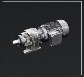
The helical inline motors have a compact design and torsionaly rigid cast iron housing. They are hygienic and have good washdown functionality due to the smooth gear casing. These gearmotors are foot mounted and available in washdown duty as well as explosion proof. The helical gearmotors are available with torque ranging from 88lb-in to 230,000lb-in.
