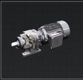
The helical inline motors have a compact design and torsionaly rigid cast iron housing. They are hygienic and have good washdown functionality due to the smooth gear casing. These gearmotors are foot mounted and available in washdown duty as well as explosion proof. The helical gearmotors are available with torque ranging from 88lb-in to 230,000lb-in.
