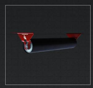
These Idlers are best used on portable conveyors and trough idler conveyors where there is not enough room to fit a traditional selt aligning idler. These use the laggaing and eccentric axles to shift under the load of the belt and track it back towards the center of the conveyor.
