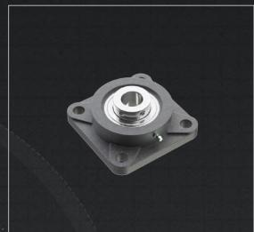
Four bolt flange bearing housings are offered in standard or corrosion resistant materials/piaint with light to heavy duty bearing inserts to meet your strength requirements. These bearings can be had with standard seals or high heat and with roller, or ball bearings as well as chrome plated or stainless steel. Four bolt flange bearings are available with standard set screw bore or eccentric locking collars.
