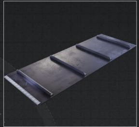
Extruded rubber and steel cleats are desired in the most industrial environments due to their low cost and durability. The bottom of cleat is concave to provide tight seal when bolted to belt. This makes repairs easy and down time less as the cleats are applied to belt with punch and wrench.
