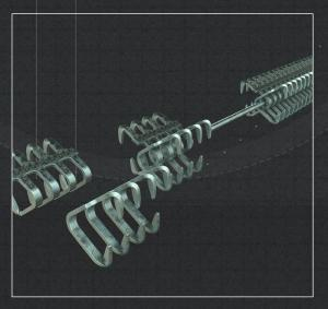
Alligator splicing is ideal for easy, economical installation of a low-profile belt splice. Available in continuous lengths, the system fits any belt width and provides uniform tension across the full belt width. Minimum pulley diameters range from 1 inch to 14 inches. Installation can be done with mechanical tooling or a hammer.
