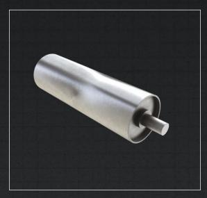
Fluent Conveyors provides flat drum pulleys with standard dimensions of 4" to 60" diameter and face widths up to 72". These pulley are available without lagging if that is necessary for your application. The crowned drum pulleys can be had with XD, QD, TL, and KLD hub configurations in nearly any bore you need.
