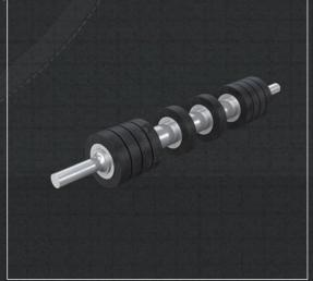
Fluent provides rubber disc rollers designed for the toughest of environments. These are made with vulcanized 60 durometer rubber discs to help reduce material build up and allow for a long life of the roller.
