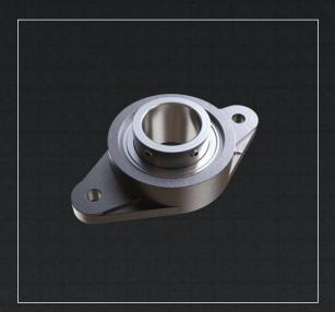
Two bolt flange bearing housings are offered in standard or corrosion resistant materials/paints with light to heavy duty bearing inserts to meet your strength requirements. These bearings can be had with standard seals or high heat and with roller, or ball bearings as well as chrome plated or stainless steel. Two bolt flange bearings are available with standard set screw bore or eccentric locking collars.
