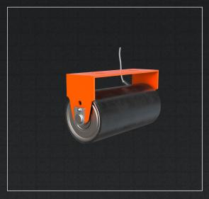
These Idlers are best used on portable conveyors and trough idler conveyors where there is not enough room to fit a traditional self aligning idler. These use the lagging and eccentric axles to shift under the load of the belt and track it back towards the center of the conveyor.
