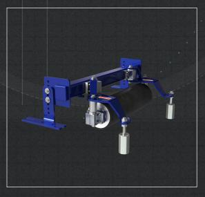
Our Pro Trainer idlers work differently from standard trainer idlers. These fit on the return side of the belt, however, the roll remains on the clean side of the belt. This reduces build up and allows for improved tracking.
