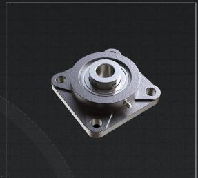
Four bolt flange bearing housings are offered in standard or corrosion resistant materials/paints with light to heavy duty bearing inserts to meet your strength requirements. These bearings can be had with standard seals or high heat and with roller, or ball bearings as well as chrome plated or stainless steel. Four bolt flange bearings are available with standard set screw bore or eccentric locking collars.
